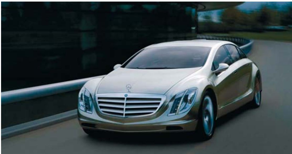
Fig. 3. Mercedes-Benz F700 concept car combining HCCI engine with hybrid-electric drivetrain [10]
